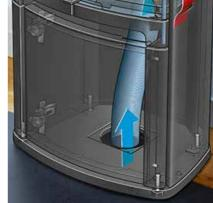
Supply air connection. Draws air in from the outside. Suitable for modern homes with a ventilation system and negative indoor air pressure.
