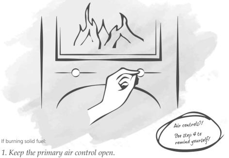
2. Close the secondary air control almost completely.
