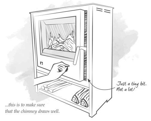
*After* 5 – 10 *minutes the draw from the chimney should be well established.*
